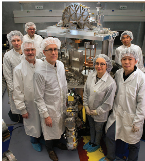
FIGURE 6.3.1 The NIST-4 Kibble balance, where the weight of a test mass is offset by a force produced when an electrical current is run through a coil of wire immersed in a surrounding magnetic field. As of May 20, 2019, it uses the defining fundamental constants that form the foundation of the International System of Units (SI) to realize the kilogram. The science team consists of, from left to right in front, Frank Seifert, David Newell, Jon Pratt, Darine Haddad, and Shisong Li. In back, Stephan Schlamminger (left) and Leon Chao (right). SOURCE: National Institute of Standards and Technology, “Watt Balance Team,” https://www.nist.gov/image/wattbalancegroupapril2016-2500pxresizedjpg ; courtesy of J. Lee/NIST.
