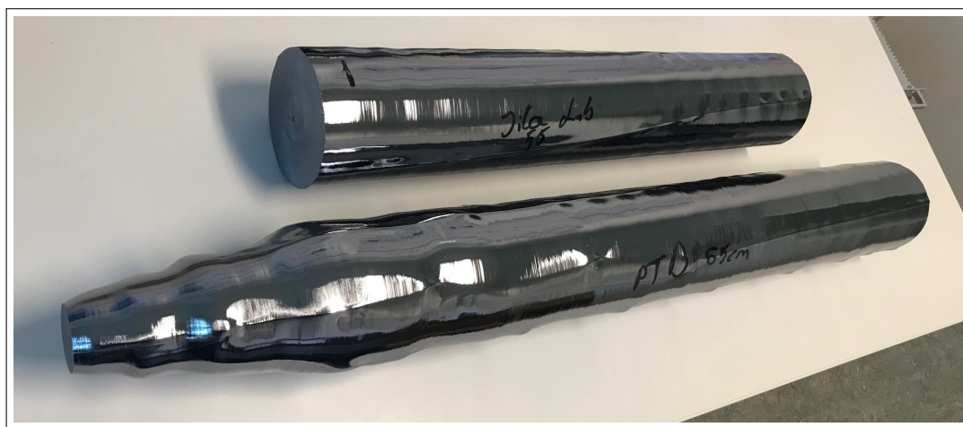
Figure 3.4: Two 55 cm silicon ingots grown at IKZ Berlin. Image courtesy of Thomas Legero.
