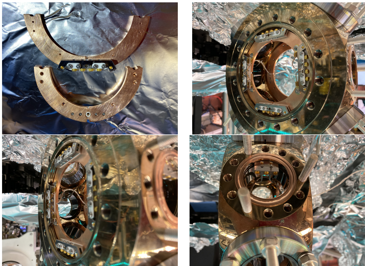
Figure 4.7: DC Stark plate construction. Top left: Example of a quadrant plate split in half, showing groove grabber assembly for both assembling all four quadrants together and mounting to the chamber. Note the use of alumina to electrically isolate each quadrant. Top right, bottom left: Picture of the plates installed into the Kimball Physics chamber, showing wiring. Bottom right: Assembly for routing quadrant plate wires around 2 3/4" CF port.
