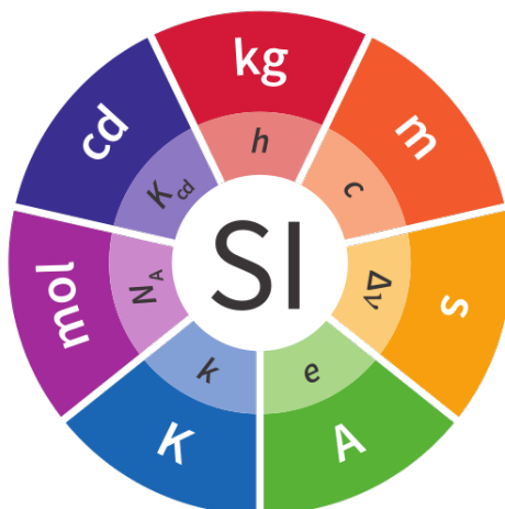
Figure 1.1: The SI Base units and defining constants. The second is defined by taking the fixed frequency for the cesium hyperfine transition \Delta\nu , the meter by defining the speed of light c , the kilogram by defining Planck's constant h , and so forth. All other units are derived from these seven base units.
