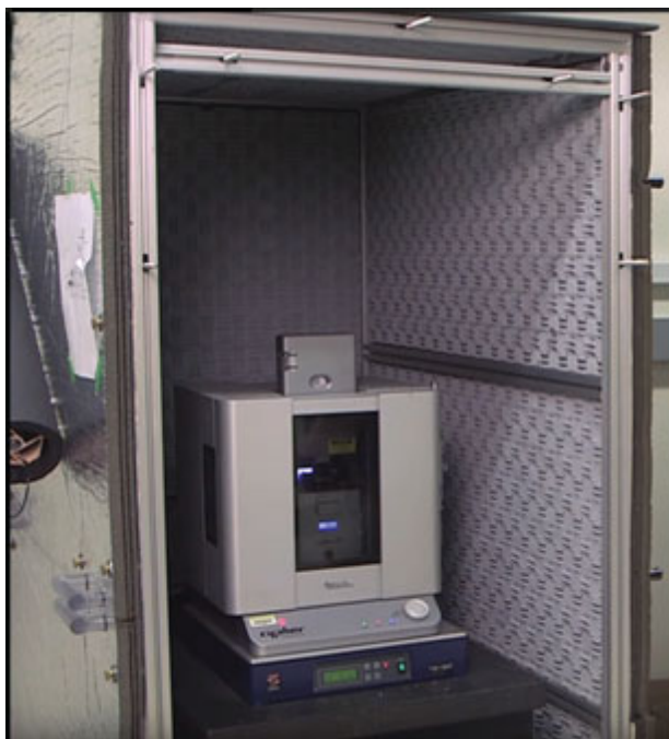
Figure 2-7: Noise isolation box around the Cypher AFM, with the front panel removed. The panels are constructed of different foams with contrasting densities, making them non-transmissive to noise. Quiet computer fans and foam tubing were installed to maintain reasonable temperatures within the box when closed. Photo adapted from (86).
