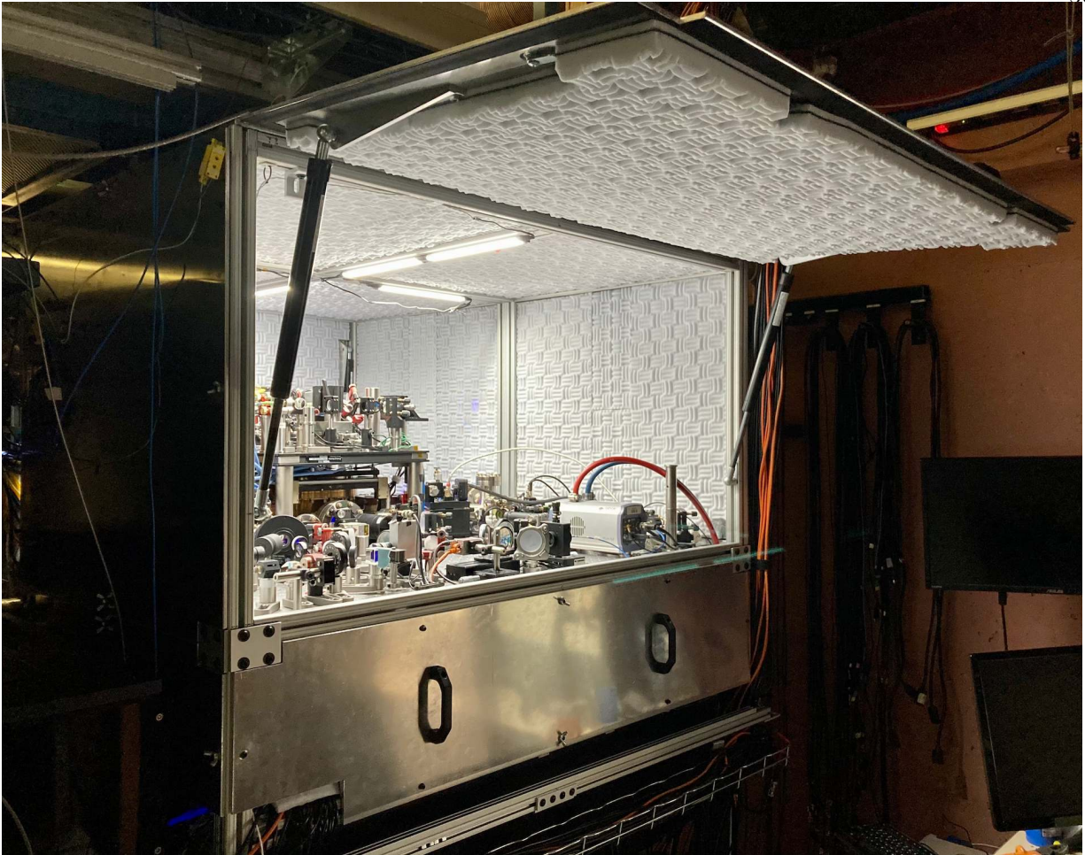
Figure 3.4: One side of the Al enclosure that surrounds the main experiment.
