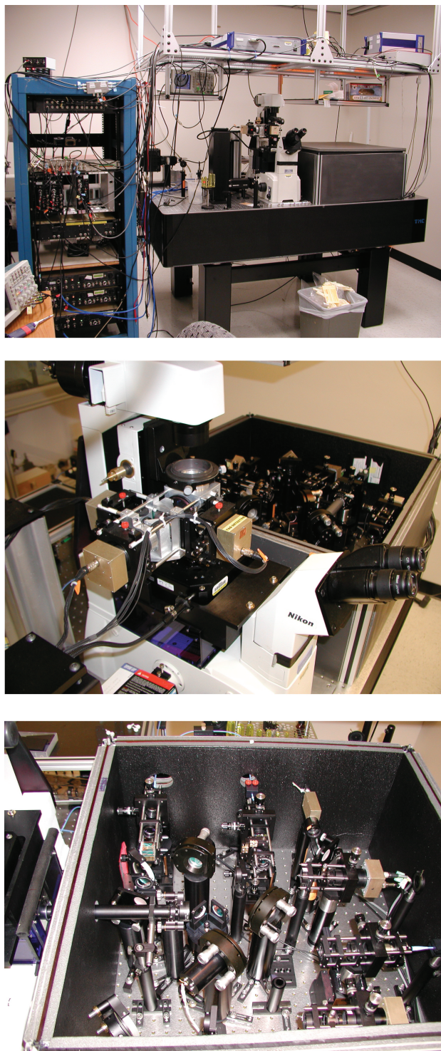
Figure 2.2: Pictures of the optical trapping microscope. Top. Optical trapping instrument. Middle. Zoom-in of the microscope and detector arm. Bottom. Zoom-in of the laser optics before the microscope.
