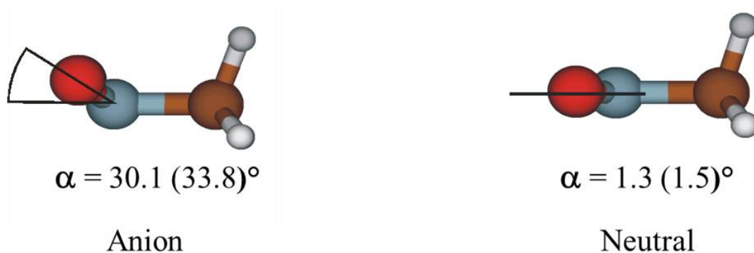
Figure 4.1 – Geometries of CH 3 NO 2 - and CH 3 NO 2 ; \alpha denotes the angle between the ONO plane and the CN bond axis from DFT calculations; results from the CCSD(T) calculations are in parentheses.
