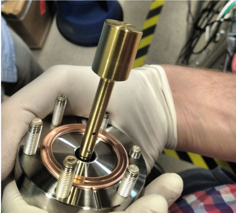
Figure 7.1: A microwave free space coupling probe used for addressing OH molecules even in the midst of the Stark decelerator. The brass structure is in good mechanical and electrical contact with the center pin of a coaxial vacuum feedthrough mounted in a 2.75" conflat vacuum connector. This is achieved with the 0-80 setscrew just visible towards the base of the brass structure. The thin region of the Brass structure has a 1/4" diameter, and the thick region is closer to 3/4" diameter.
