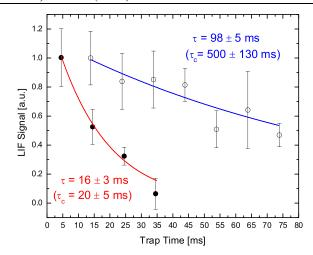
FIG. 4 (color online). Measured ( $\tau$ ) and deconvolved collisional ( $\tau_c$ ) lifetimes of magnetically trapped OH at a background pressure of  $1 \times 10^{-6}$  Torr ( $\bullet$ ) and  $4 \times 10^{-8}$  Torr ( $\bigcirc$ ).
