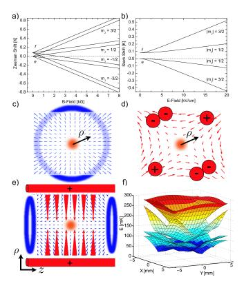
FIG. 2 (color online). (a) Zeeman and (b) Stark effects of the ground state structure of OH. (c) Magnetic and (d) electric quadruple fields viewed from  $\hat{z}$ . (e) Side view of the MET configuration with quadrupole E and B fields. (f) Transverse adiabatic potential surfaces for various components of the OH ground state at the longitudinal MET center. The top surface depicts the decelerated and trapped  $|J = \frac{3}{2}, m_J = \frac{3}{2}\rangle$  state.
