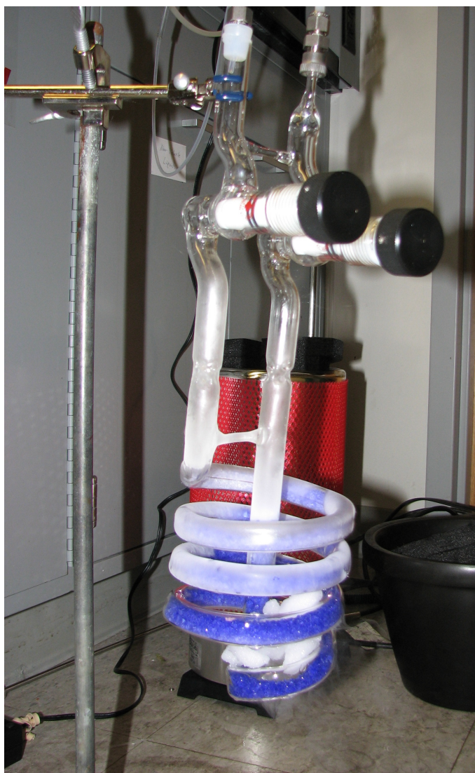
Figure 8.12: Photograph of the ozone trap. Silica gel provides a porous surface and provides a means to trap generated ozone. The dark blue color indicates a high concentration. The trap is stored with dry ice to produce a lower vapor pressure as well as to prevent spontaneous combustion.
