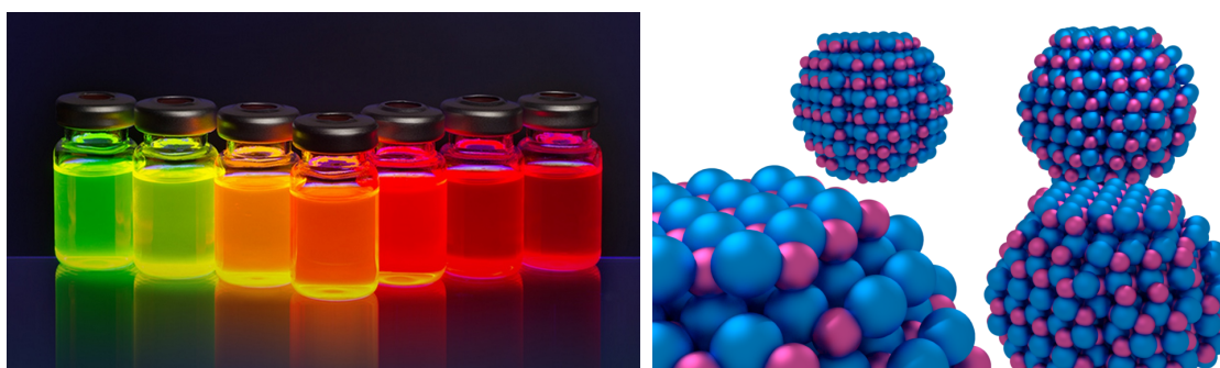
Figure 1.2: Cadmium selenide quantum dots (CdSe QDs) . (left) Each vial contains the same chemical composition (CdSe QDs and toluene), but the different sizes cause the nanocrystals to fluoresce different colors. The bandgap increases with decreasing particle size, so the vials on the left contain the smallest QDs (largest bandgap) and the vials on the right contain the largest QDs (smallest bandgap). Image courtesy of NN-Labs Inc. (right) An illustration of CdSe quantum dots shows the individual atoms clustered into faceted nanocrystals.
