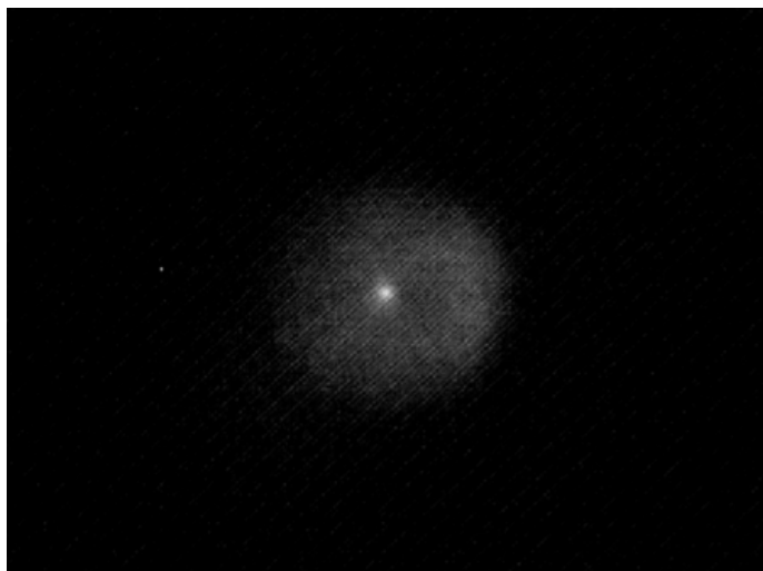
Figure 2.11: Representative VMI image of the photoelectron momentum distribution from a sample of 2.3 nm diameter CdSe quantum dots taken at t=100 fs. The center of the image corresponds to zero momentum, with electron energy/momentum increasing radially outward, and the laser polarization is in the vertical direction. The slight left-right asymmetry is due to detector inhomogeneities. This image has been background subtracted to remove contributions due to scattered light and the ionization of the hexane solvent and helium carrier gas. Figure from [79].
