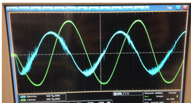
Figure 5.16: 50 shots at a 1 Hz repetition rate of \pm 12 kV output at 5 kHz using an amplifier filled with SF 6 . The output voltage is shown in green and the output current as measured across the sense resistor is shown in blue.
