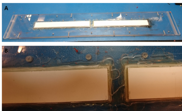
Figure 5.21: The interior insulating polycarbonate wall with boron nitride inserts. Each side wall uses two boron nitride pieces (A). The black scorch mark on the right-hand side shown a point where the wall failed. A close up of the inset boron nitride (B) shows the step that increases the path length between the aluminum wall and the back plane of the FET.
