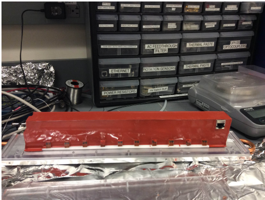
(a) Potted amplifier bank immediately after it is released from the mold.
