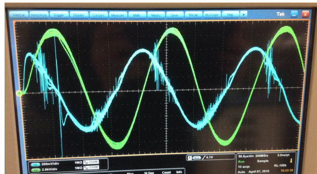
Figure 5.20: Current (blue) dips caused by proximity to polycarbonate. Usually current oscillations do not affect the voltage (green) on the decelerator, but when the current issues are severe enough they also cause droops and bumps in the output voltage.
