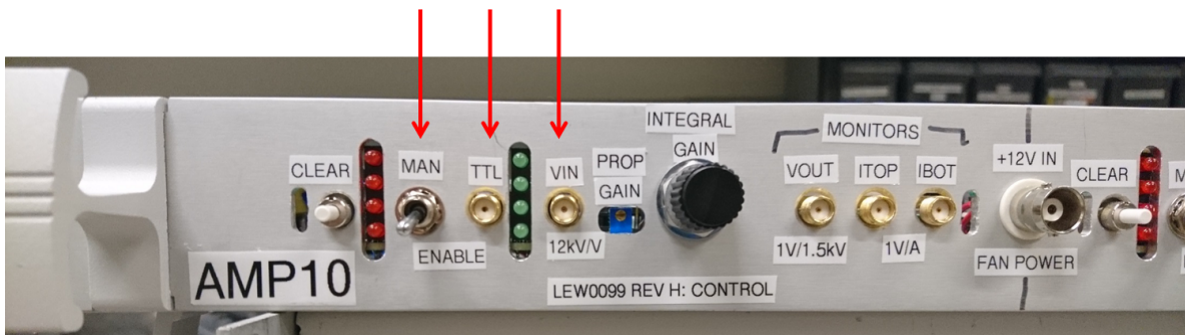
Figure 5.11: The front panel of the amplifier control box. The manual enable switch, TTL enable SMA input, and V_{in} SMA input are noted by red arrows. The manual enable switch and TTL enable SMA input together control the output state of the amplifier. The desired chirped sinewave control signal is set via the V_{in} SMA input.
