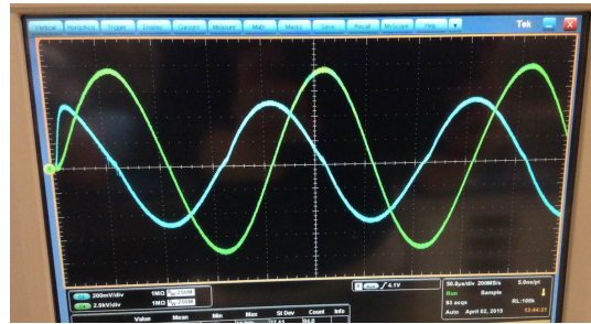
(b) With the addition of SF 6 the current oscillation issue is almost entirely suppressed.
