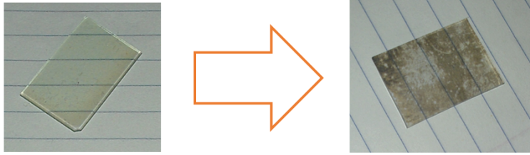
Figure 8.27: Images of an ITO-coated plate before and after exposure to a high K flux.
