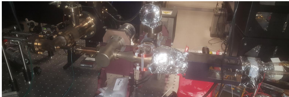
Figure 2.6: The old vacuum chamber in the first generation KRb experiment. The vapor cell MOT area is on the right, and separated by a large differential pumping section and a gate valve is the science cell side.
