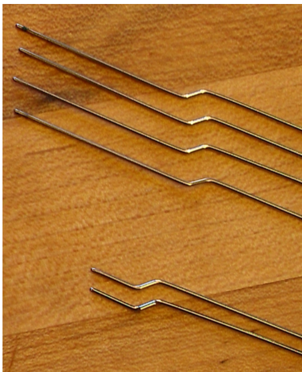
Figure 8.14: Tungsten rods bent to go into the science cell. The top four rods go between the ITO-coated plates, and the bottom two will be faced off to contact the plates. This image was taken after the rod tips were rounded, but before any cleaning.
