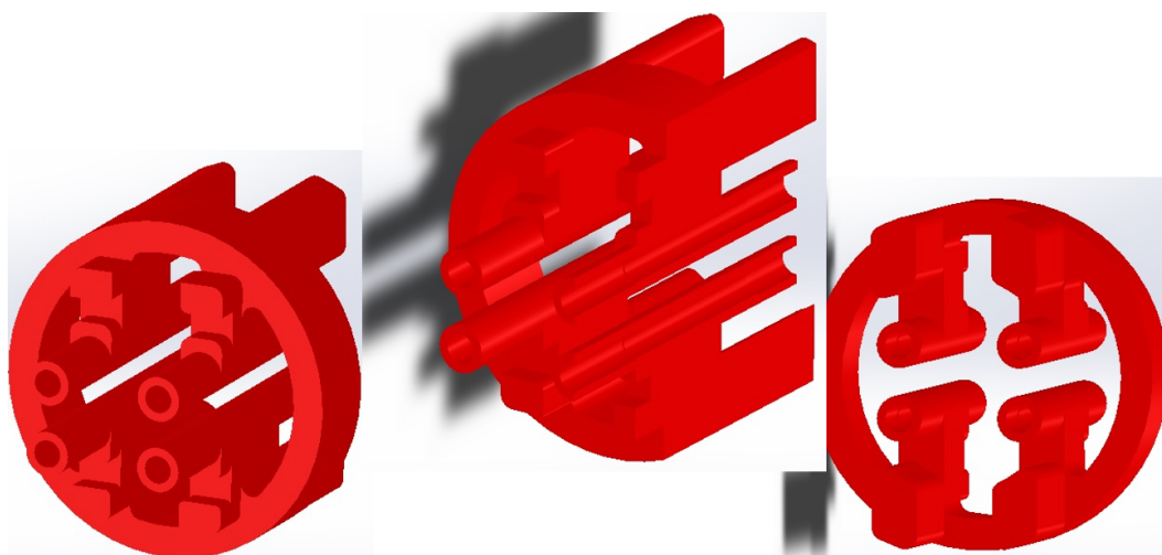
Figure 7.3: The front macor holder in the science cell. The hole diameter for the rods is 1 mm, and the entire diameter is \approx 15 mm. The groove on the front side holds the ITO-coated plates.
