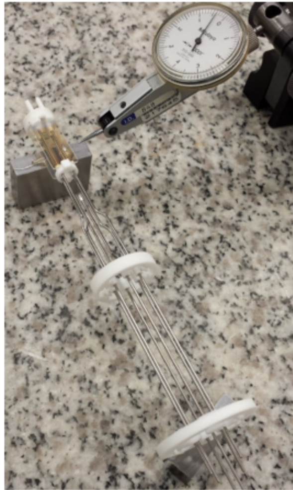
Figure 8.16: Measuring the angles between the rod and plate electrodes. A dial indicator on a super-polished granite block was swept along the length of the rods and plates to measure their relative angles.
