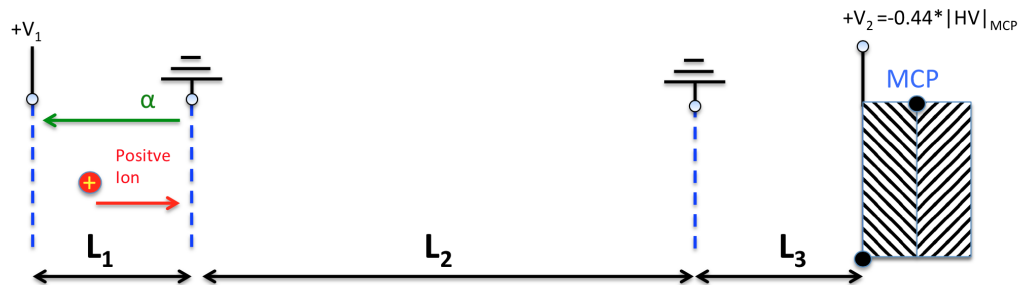
Figure 6.12: Schematic of different regions and voltages used to describe a generic two-electrode TOFMS, the free flight region for mass separation, and a MCP ion detector with a repeller grid.
