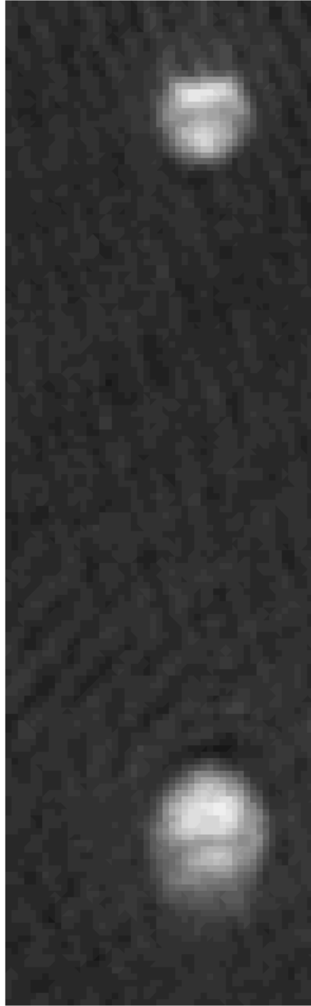
Figure 4.5: Image of both the |2, 1\rangle (top) and |1, -1\rangle (bottom) condensates after dropped from the magnetic trap. In the trap the |2, 1\rangle sits below the |1, -1\rangle .
